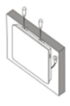
Tighten the two screws on the top of the bracket, ensuring the unit is secure, before connecting the power.
