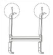
Unscrew the two screws holding the wall mounting bracket to the back of the body, and keep in a safe place to allow the option of wall mounting in the future.
